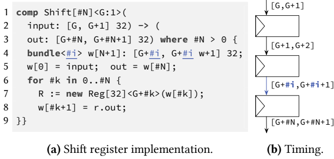
Figure 6. A shift register implementation in Lilac and a block diagram visualizing the timing of each bundle wire.
